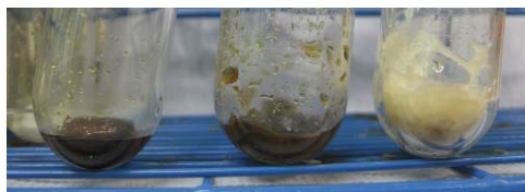
Fig. 5 Dry pine specimens treated at 120 °C for 15 h with [C_4C_1im][Me_2PO_4] (left), [C_4C_1im][MeCO_2] (middle) and [C_4C_1im]Cl (right).
